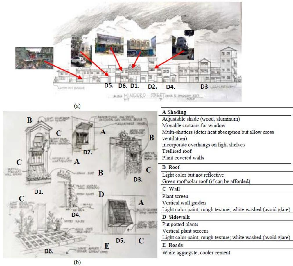
**Figure 13** (a) Elevation of identified houses where strategies can be applied to the area
