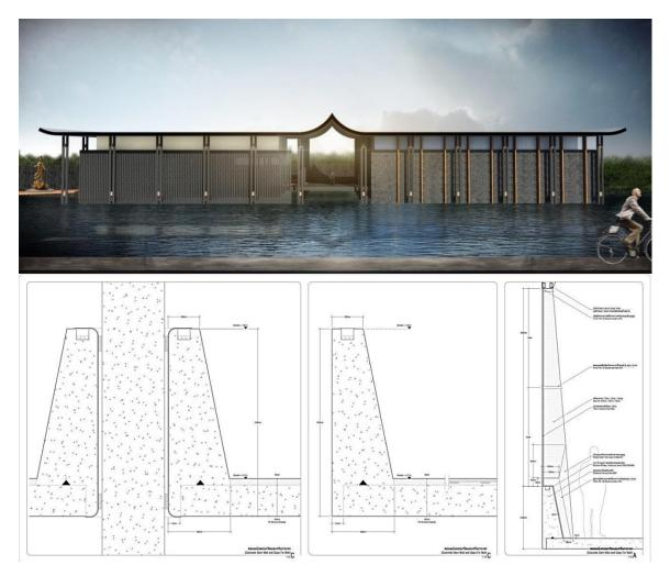
The exhibition space was designed as a floor slab with a tapered concrete perimeter wall and collars around each internal column.
