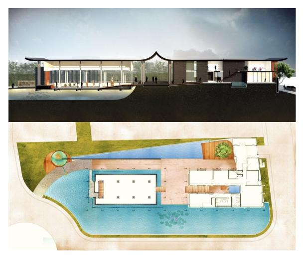
Given the scale and complexity of the program and the risk involved, it was decided early on with the structural engineer that only one mass needed to float. The exhibition hall is essentially a large, open volume, and its contents are temporary. It was the better candidate for experimentation precisely because it didn't really need to float.
